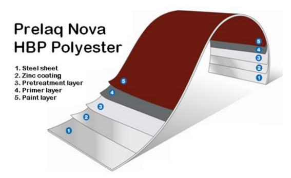
Prelaq Nova is a special extra-thick variant of polyester coating. It has a wear-resistant, textured surface achieved by polymer grains being mixed into the paint. It also has better forming properties than ordinary polyester.
