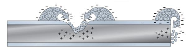
The zinc coating provides the sheet steel with double protection against corrosion. It serves as an effective barrier that excludes oxygen and moisture, and it provides cathodic protection at cut edges and at any point where the zinc coating has been damaged.
