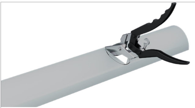
Split the cut edges with a chisel or pliers to gain access with the sheet metal shears. Use a pair of metal shears to cut the edge of the hole.
