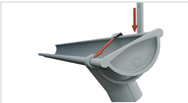
If the fascia sheet is not in place, it is easiest to insert the gutter in the front edge of the bracket first.
