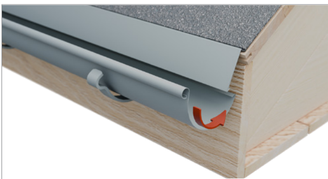
If the fascia sheet is in place, it is easiest to first insert the gutter in the rear edge of the bracket under the fascia sheet or rigid felt support tray.
