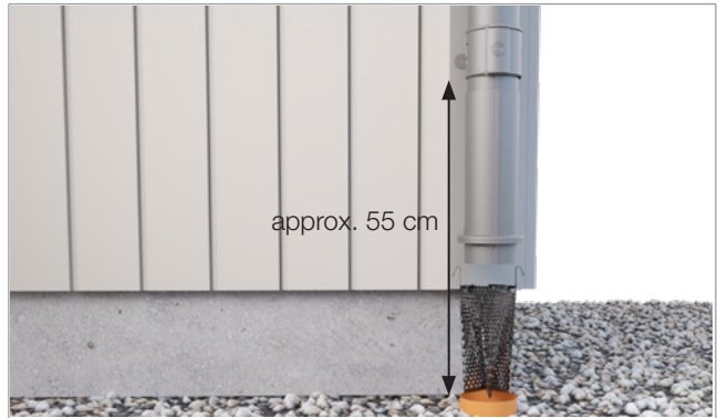
The BUTK drain shoe is easily moved up the downpipe. The drain shoe is supplemented with a leaf strainer to prevent blockage of the ground pipe. A DVSIL storm water strainer is hidden inside the ground pipe. Bear in mind that the bottom pipe holder must be high enough to be able to move the BUTK up and lift out the strainer for cleaning.
