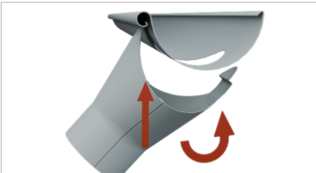
Insert the edge of the outlet into the bead of the gutter at the front edge.
